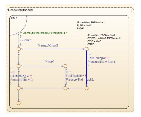
You can avoid the **Out of bounds array index** in several ways. One way is to constrain the input variable index using a Saturation block before the Stateflow chart.
